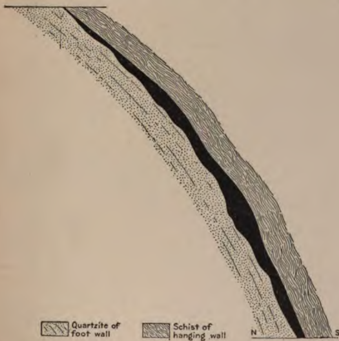
FIG. 155.—IDEALIZED VERTICAL NORTH-SOUTH SECTION, FERRIS-HAGGARTY MINE, ACROSS THE OREBODY, SHOWING CONVEXITY AND IRREGULAR DIP, (SPENCER)
